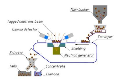
Fig. 1. General scheme of the setup.
