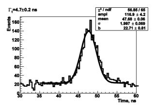
Fig.6. Time spectrum of  $\alpha$ - $\gamma$  coincidence for carbon sample for coincidence between  $\gamma$ -channel No and  $\alpha$ -channel No approximated by a Gaussian and flat background.
