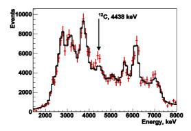
Fig.8. Gamma-ray spectrum 8 mm diamond imitator in 50 mm kimberlite ore (left). Similar figure for 14 mm diamond imitator in 160×90×90 mm kimberlite ore rock (right). Red points with error bars represent gamma-ray spectrum for tagged beam irradiating diamond simulant location. Black histogram represents spectrum of ore sample averaged over all tagged neutron beams.
