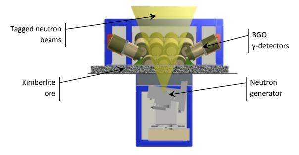
Fig. 2. General scheme of the neutron module.
