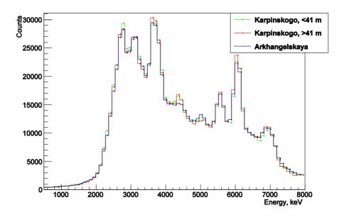
Fig.7. Energy spectra of investigated core samples from different sources shown in red, green and blue.
